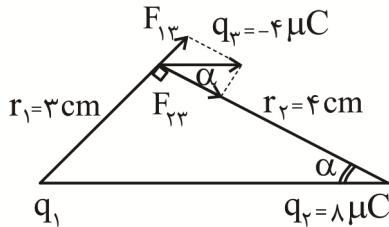
$$\tan \alpha = \frac{r_1}{r_2} \rightarrow \frac{3}{4} = \frac{F_{13}}{F_{23}} = \frac{\frac{k |q_1| |q_3|}{r_{13}^2}}{\frac{k |q_2| |q_3|}{r_{23}^2}}$$
